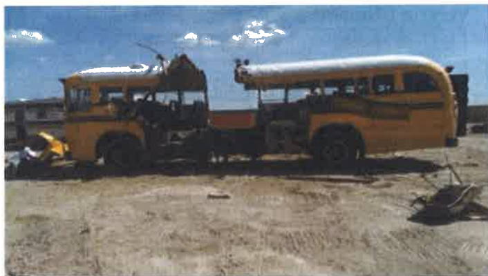
Example of acceptable destruction of vehicle chassis
