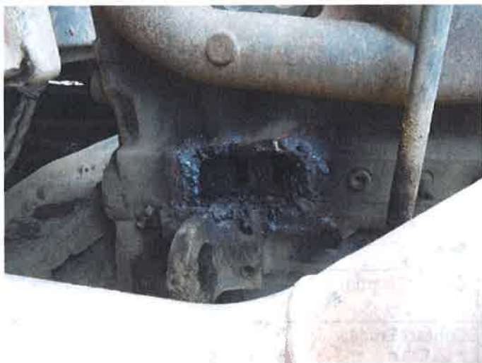
Engine: 5" hole in engine block
