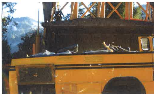
Example of acceptable destruction of vehicle chassis
